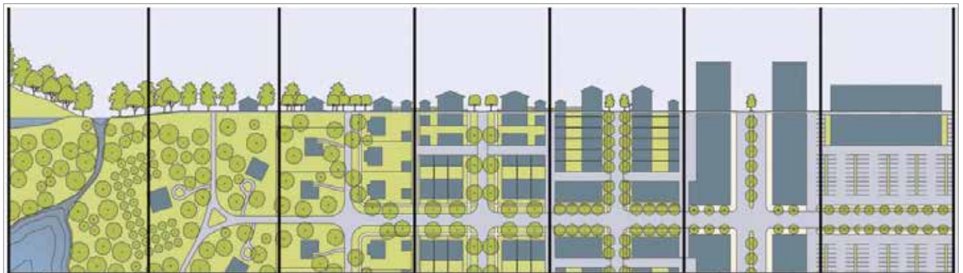
Figure 4.2: Transect Zones from Natural (left) to Special District (right) Source: Duany Plater-Zyberk & Company
