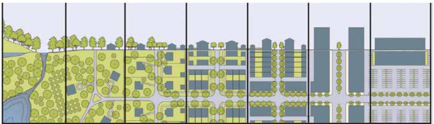
Figure 4.3: Transect Zones from Natural (left) to Special District (right) Source: Duany Plater-Zyberk & Company
